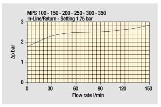
Bypass valve pressure drop
