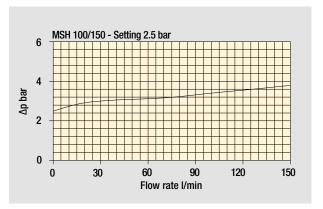
Bypass valve pressure drop
