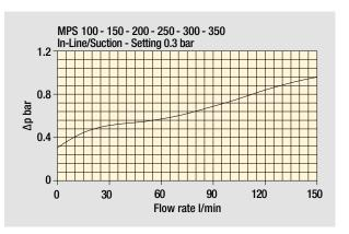
The curves are plotted using mineral oil with density of  $0.86 \text{ kg/dm}^3$  in compliance with ISO 3968.  $\Delta p$  varies proportionally with density.
