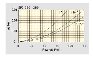
Bypass valve pressure drop
