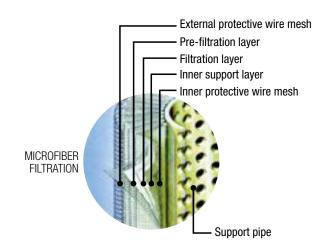
The filtration efficiency of metallic mesh filtrations is defined as the maximum particle size that can pass through the meshes of the filtering grid.
