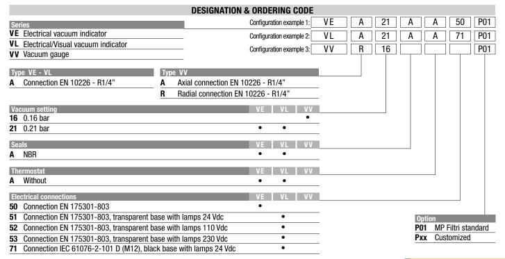
Clogging indicators are devices that check the life time of the filter elements. They measure the pressure drop through the filter element directly connected to the filter housing.
