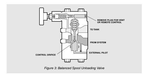
These valves are commonly used in "Hi-Lo" circuits. Combined two-pump output is supplied to the system until the load reaches the pre-set pressure setting of the unloading valve. Pilot pressure then opens the valve and delivery from the high
